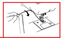
Draw the threads up and into the thread cutter. The threads are cut the proper length for starting the next seam.
